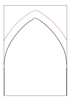
Don't cut the red line! It just shows where the bricks for the outermost arch need to be cut in.
