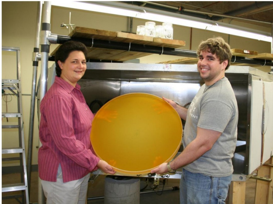
Lisa and her student, Kevin, holding a 25 inch epoxy mirror. The oven for spinning 2-meter mirrors is in the background.
