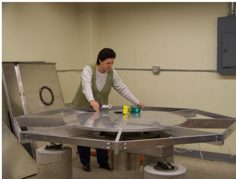
Lisa assembling the arms on the platter for spin-casting 2-meter epoxy mirrors. The oven panels with heating elements can be seen in the background.
