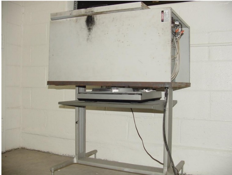
First generations epoxy mirrors were manufactured on a record turntable using a conventional electric lab oven for the heat source.
