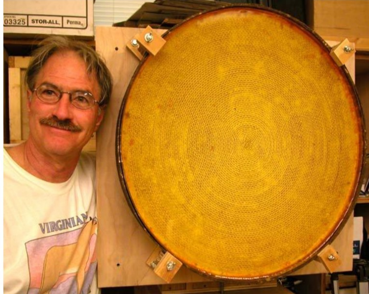
Terry in the optics lab preparing to test a 0.5 meter epoxy mirror.
