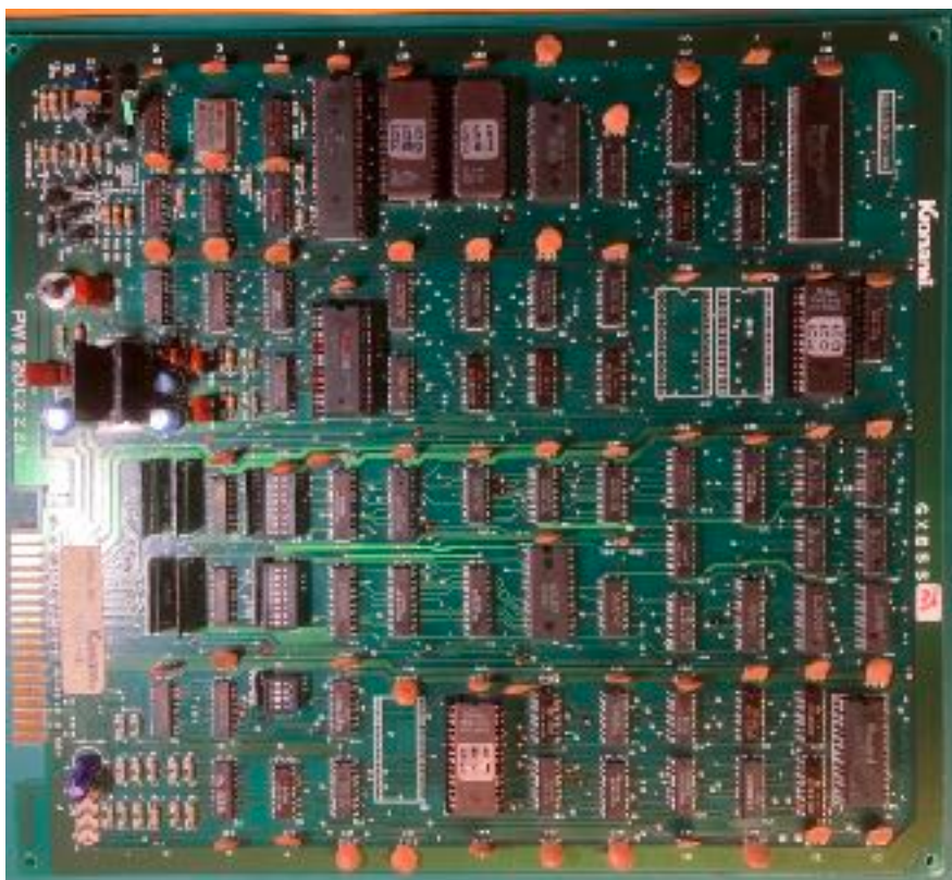
The PCB with the two 28-DIP daughter boards removed
